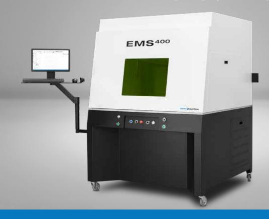
With the ability to run up to four axes, EMS400 is ideal for large tray and part marking. EMS400 features an automated 24" x 24" XY stage (610mm x 610mm), ideal for marking trays of parts or large components in multiple locations. A front vertical pneumatically actuated door maximizes operator ergonomics.
